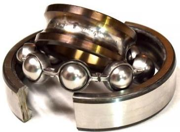
When bearings operate in a clean environment, the primary cause of damage is the eventual fatigue of the surfaces where rolling contact occurs. However, when particulate contamination enters the bearing system, it is likely to cause damage such as bruising which can shorten bearing life dramatically.
