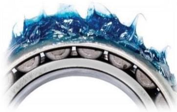
All greases are not compatible with one another, and if mixed, can cause failure, due to changes in consistency, abnormal oil separation, changes in drop point, shear stability, as well as possible additive incompatibilities.
