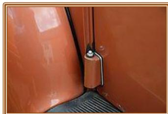
[A Grease Nipple on the Driver's Door of a 1956 VW Beetle](#)
