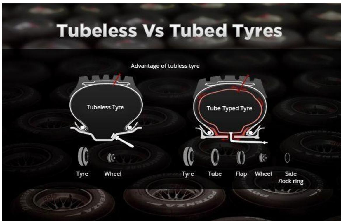
Also, since a tubed tyre has more components (tyre, tube, rim) compared to a tubeless tyre (just tyre and rim), performance and efficiency are better with a tubeless tyre.
