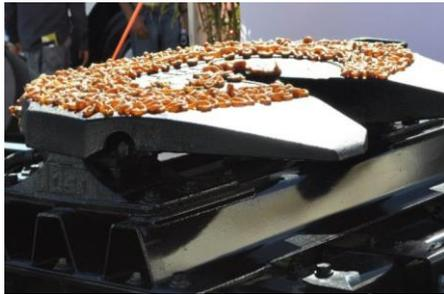
The correct spec grease for a heavy-duty truck fifth wheel coupling is an EP2 (extreme pressure) black, sticky, graphite impregnated grease. And only a small cupful of EP2 grease matches the task. The picture here is an environmental horror that gets swept off the fifth wheel falling into the truck chassis and eventually the road surface, which in turn creates slippery patches and road safety hazards. It's all about friction.....in the coupling and on the road.
