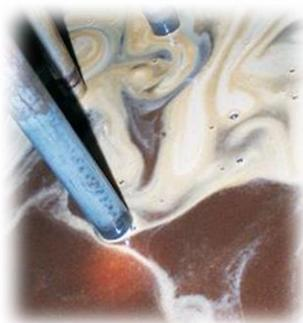
Lubricant foam has a low load carrying ability. Excessive foam build-up in a reservoir or sump will rapidly lead to excessive wear and catastrophic failure of the system. (Noria.com)
